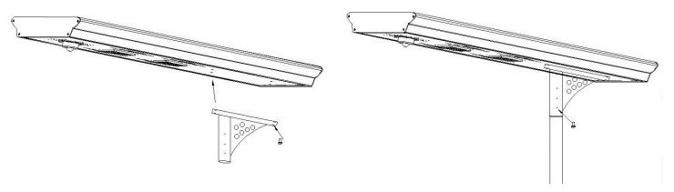
Use 4 screws to fix the fitting support on the lamp and fix the lamp on the pole with screws.
