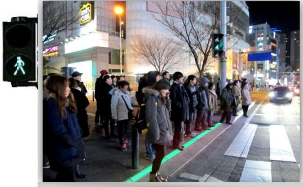
Corresponding with go signal of existing signal system, switching on the green light means enable to cross safety.
